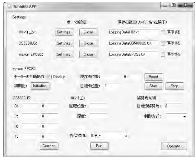
Fig. 4 Application software 'Tonai60 APP' for controlling Tonai60.
